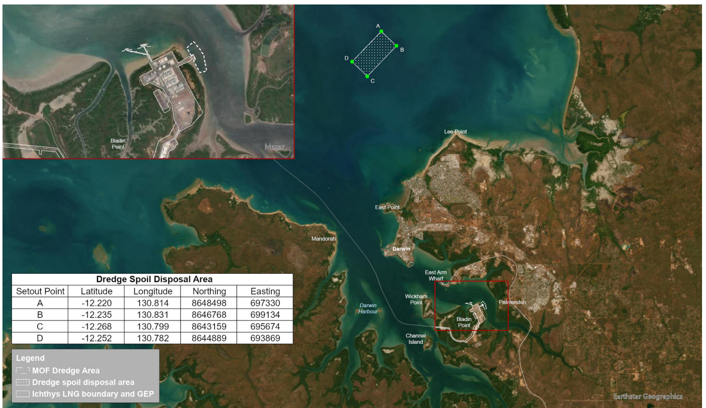
Figure 4 Minor dredging campaign location and dredge spoil disposal area.
